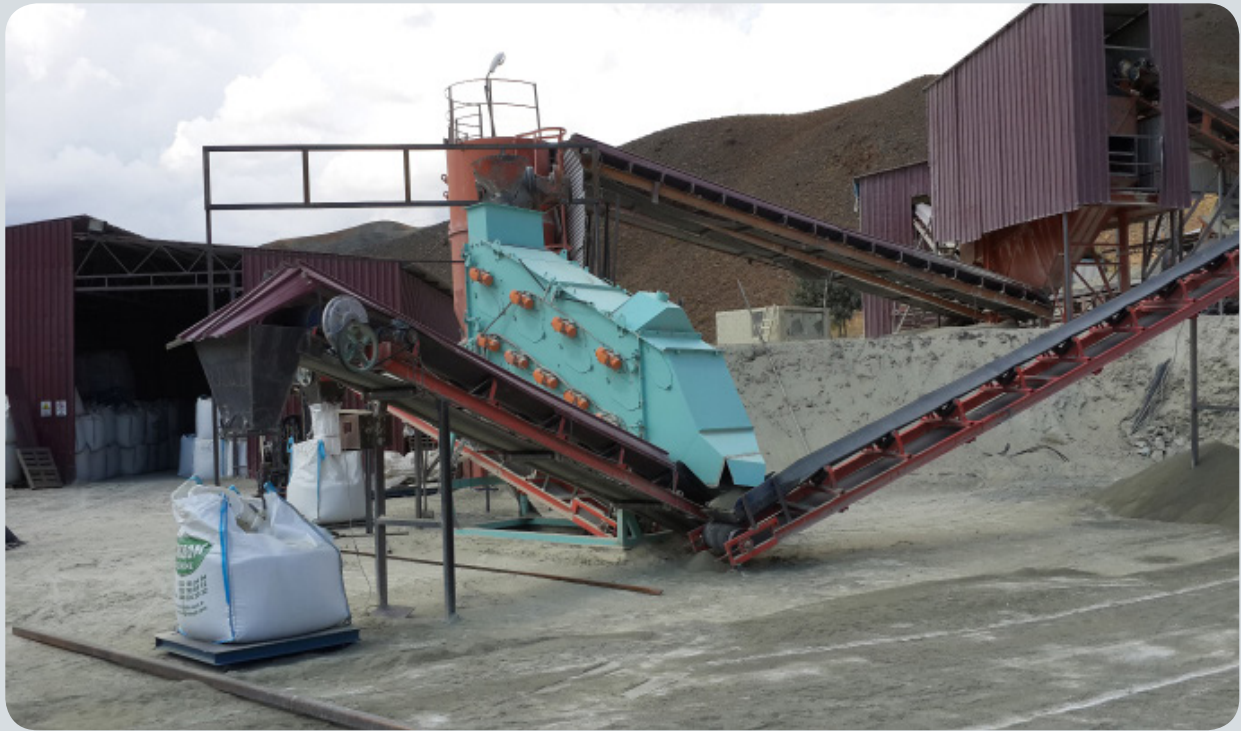
In this plant, a double decks VCR-D screening machine in size of 1000x3000 screens Olivine in 200 microns - 500 microns with a capacity of 30 tone/hour.
