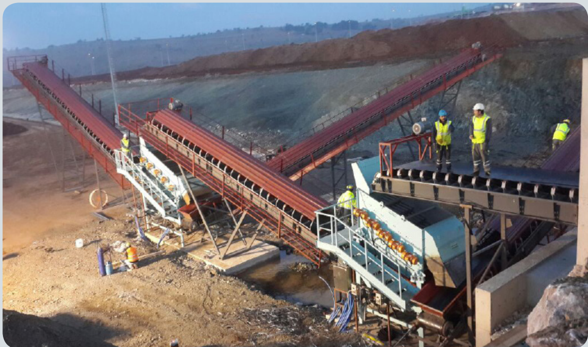
In this plant, one piece VCR-D screening machine in size of 1500x4000 and one piece VCR grill screen moisty Clay in -50 mm with a capacity of 150 tone/hour.
