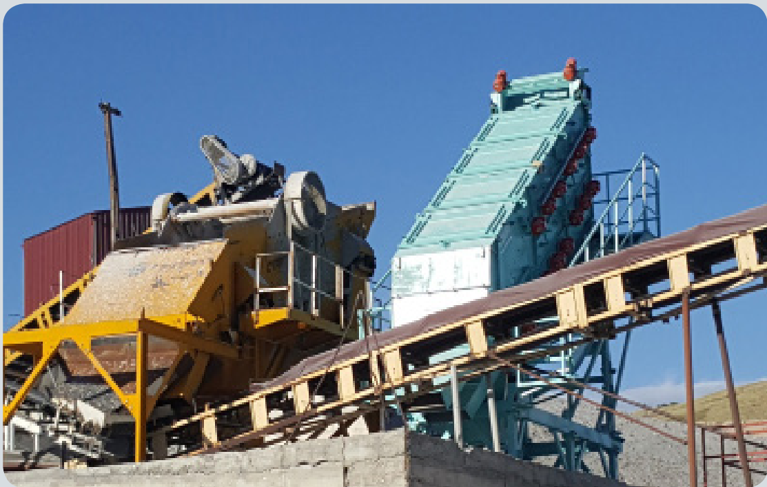
In this plant, a double decks VCR-D screening machine in size of 1500x6000 screens Natural Pearlite in 3 mm - 5 mm with a capacity of 100 tone/hour.
